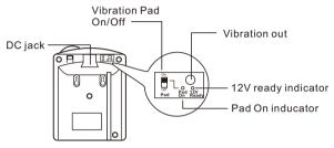
DC jack: If using the vibration pad, It must be connected a 12V 400mA AC/DC adaptor to this jack.
